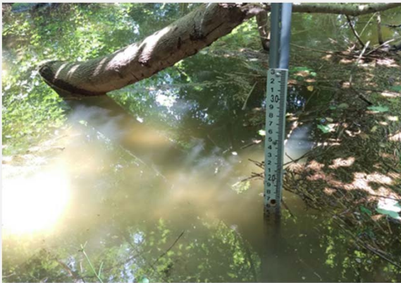
Level gage and logger housing at Site A marsh
